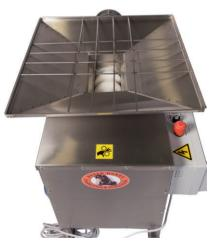
Based on feedback from beekeepers and long-time experience, we can safely say that a waxpress with production power of 100 kg/h has the most optimal power for both a novice beekeeper and a big manufacturer.
