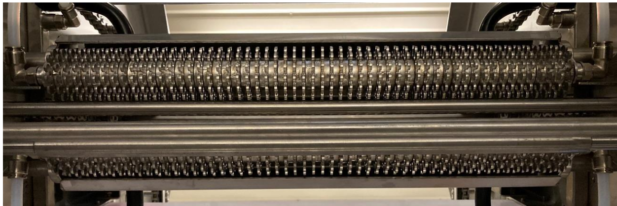
Cappings scratchers` system as seen from below the machine.
