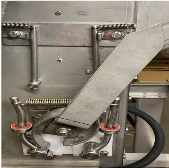
Blade gap wider - direction (right)
