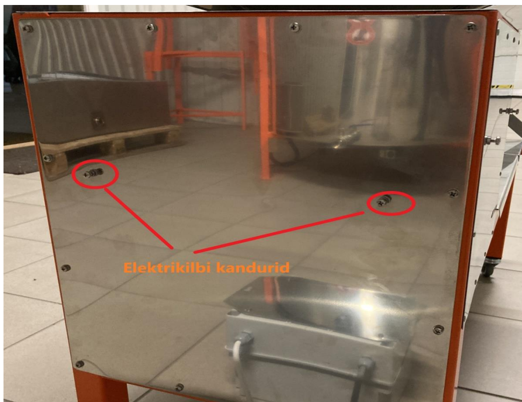
Rear end carriers for electrical panel
