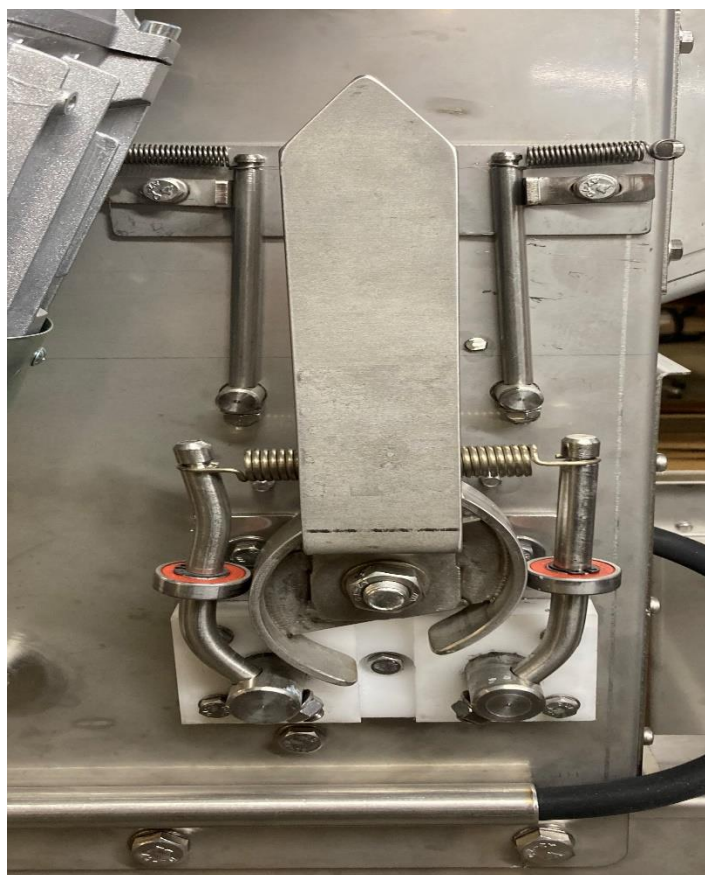
Adjustment lever of cutting knives
