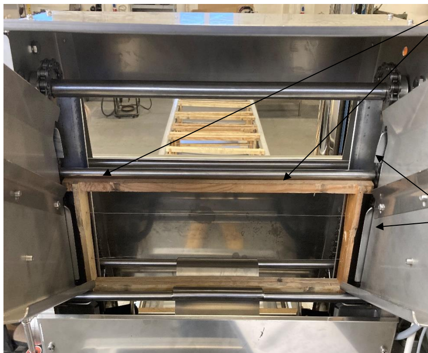
Positioning of the frame between the feeding system
