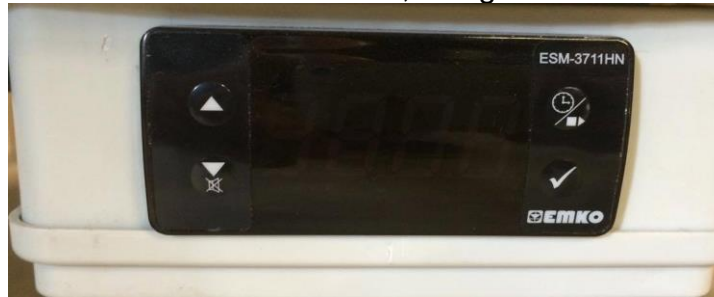
Figure 3. Temperature controller switched off
