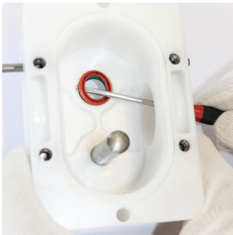
Fig. 12: Remove the red/blue shaft seal
