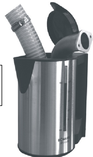
Fig. 25: Heating of hose and pipe bend
