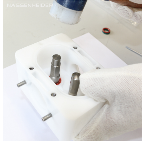
Fig. 11: Knock out the driving shaft
