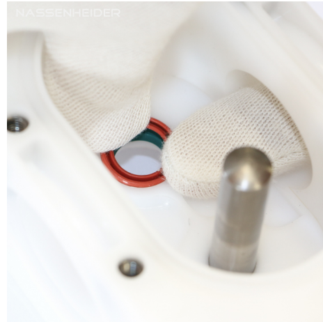
Fig. 15: Insert the red/blue, greased shaft seal
