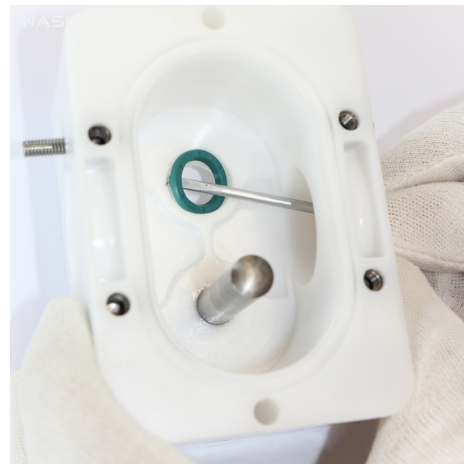
Fig. 13: Remove the green/blue shaft seal
