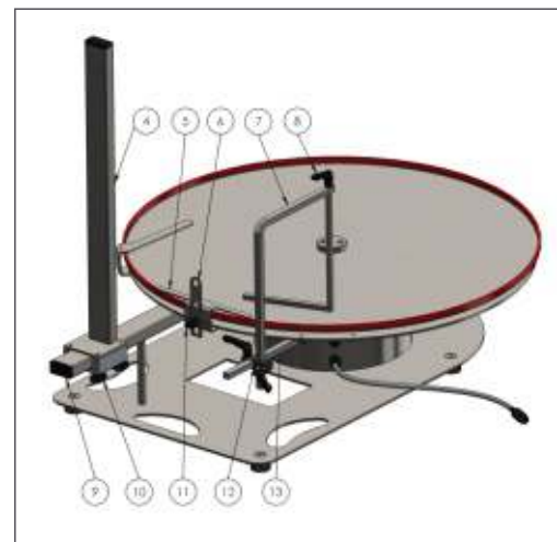
Assembly of stand, sensor holder and container guide bracket
