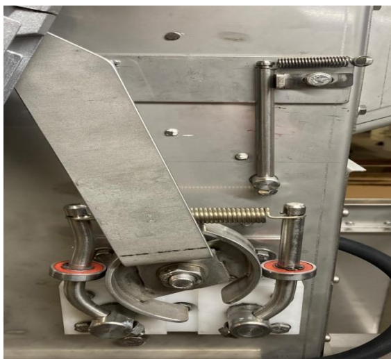
Blades gap narrower - direction (left)
