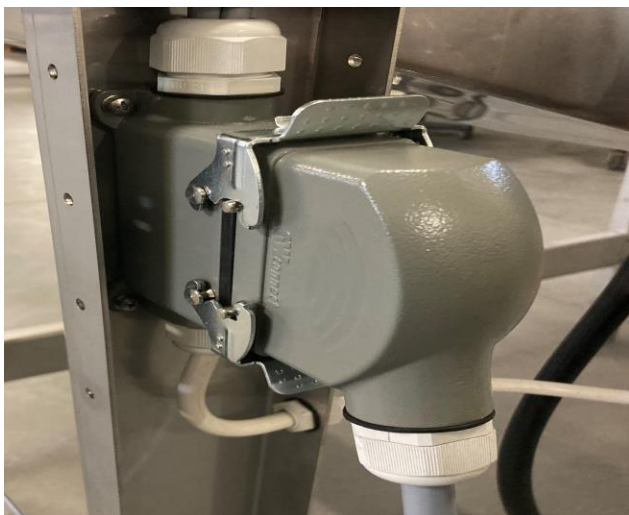
Connected and locked PIN16 connector.
