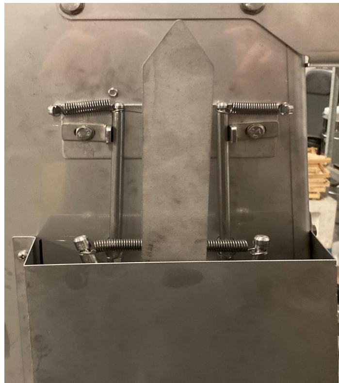
Cutting knife adjustment lever
