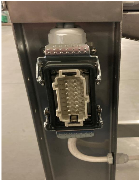
Female side of PIN16 connector.
