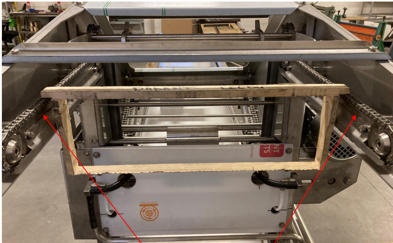
The chains of the feeder mechanism
