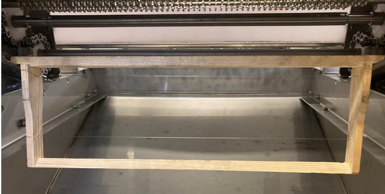
Position of the uncapped frame after uncapping in the lower part of the machine.
