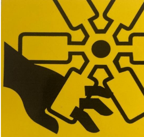
Rotating parts / risk of entanglement with machinery
