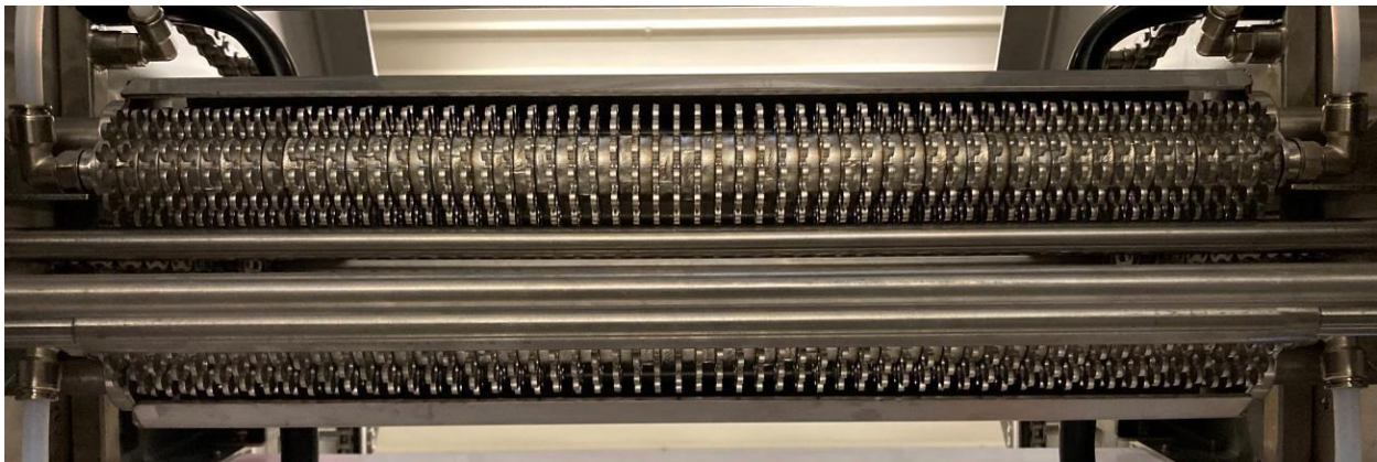
Comb loosener` system as seen from below the machine.
